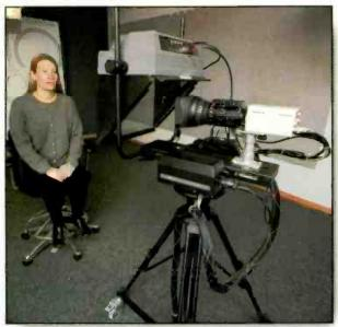
The studio's Sony DXC-950 camera with ESI robotics (shown above) was positioned by an operator in communication with broadcasters via a coordination phone line.
