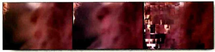
Figure 2. Lost packet in an I frame results in severe blockiness in a neighboring B frame.
