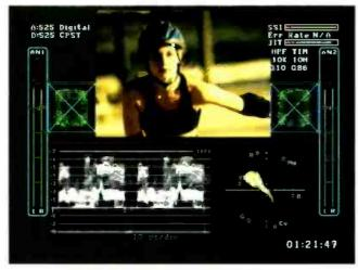
On-screen display of SD 601 input signal
